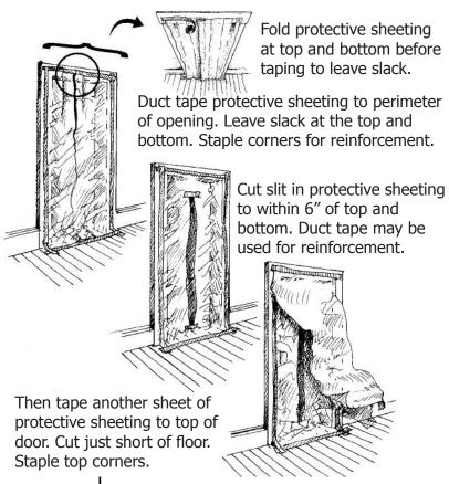
In addition to the steps outlined in the section on setting up the work area, high dust jobs require containment of doors that allow access but prevent the migration of dust.
